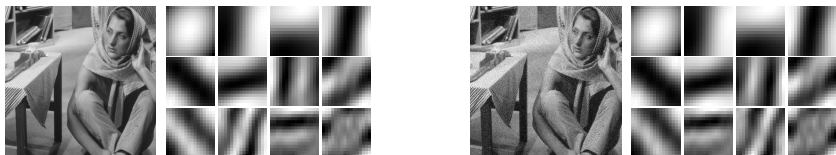
Figure: The top 12 bases learned from all 16 \times 16 patches of Barbara, both with (right) and without (left) Gaussian noise. The noisy image is produced by adding Gaussian noise to the clean image, resulting in SNR of 5.87.
