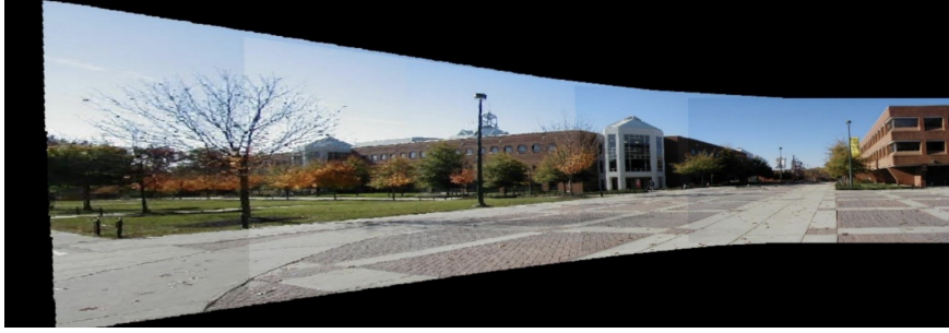
Figure 7.3: Different views related by only rotation stitched together. This also explains why we can get good panoramic photos of the wild, e.g. when on top of a mountain. It is because the distance to the plane is too far away and large d makes T negligible and H almost the same as R , making it different camera views only differ by a rotation.
