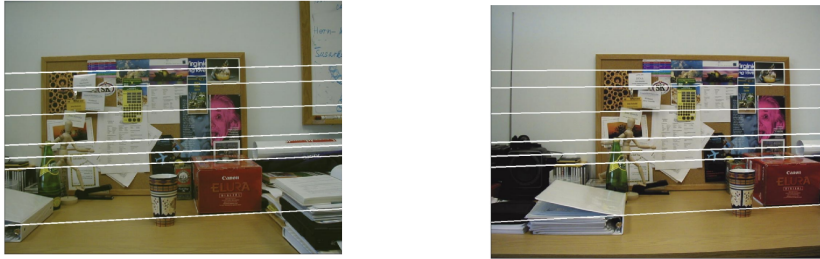
Figure 7.2: We can use epipolar geometry to tell where the corresponding image coordinate in another camera frame could lie, which are the white lines.
