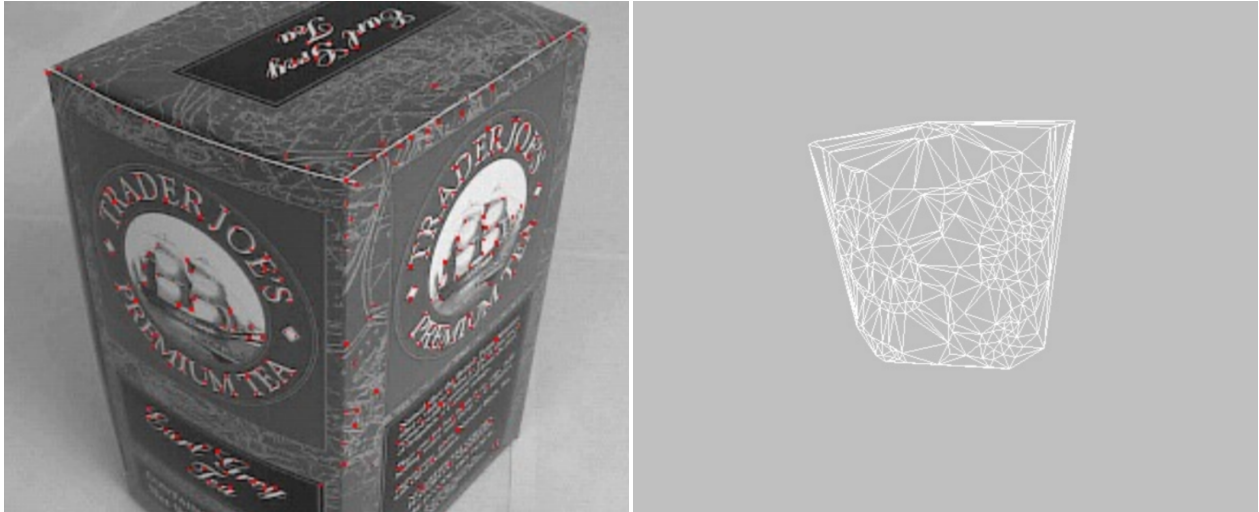
Fig:6.2.6.1 (From lecture slides) Feature Rich Image(Left) 3D Reconstruction Preview(Right)
