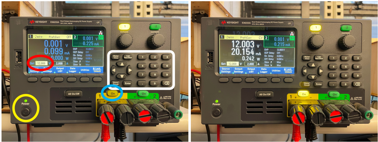
Figure 4: (Left): Power supply when turned on but output is OFF. Note the power button (yellow), the output “ON” button (blue), the set voltage (red), and the keypad(white) Right: Power supply when output is ON. Note the glowing output “ON” button.
