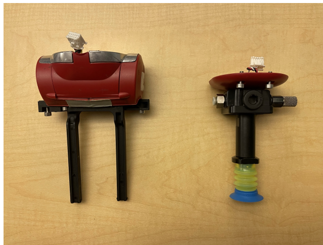
Figure 3: Electric parallel-jaw gripper (left) and pneumatic suction gripper (right).
