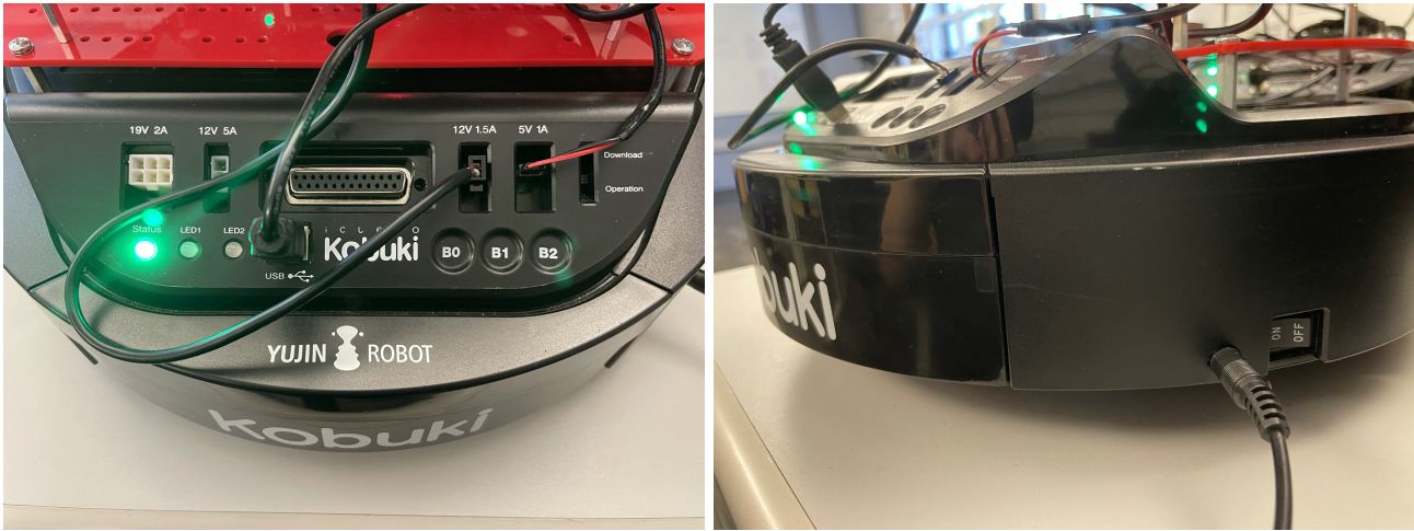
Figure 10: (Left): Status LED on Kobuki base, indicating on and high battery. (Right): Charging port and on-off switch on Kobuki base.
