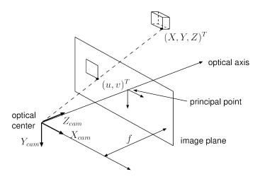
Using the image above, find the relationship between the 3D point  $(X,Y,Z)^T$  to its corresponding 2D projection (u,v) on to the imaging plane.
